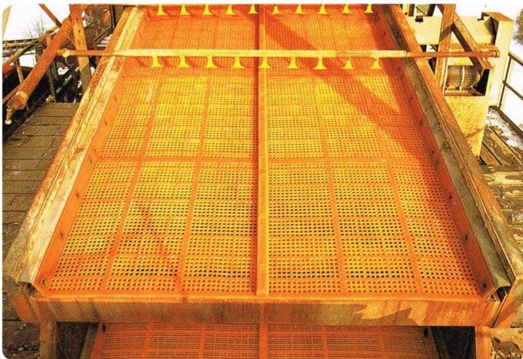
The WS85 modular panels are manufactured with integral steel reinforcement parallel to the panel width and selected for each individual application to accurately transmit the dynamic forces of the screening machine and support the bed of material.
